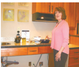
Designer Lora Creswick demonstrates her Universal Kitchen with the adjustable counter at maximum height. Notice adjustable under-counter electrical & plumbing fixtures.
